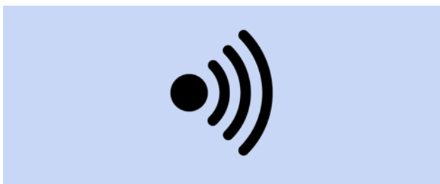
Figure 1-7 This symbol indicates the option to test a circuit for continuity, with audible feedback. It's a very useful feature.
